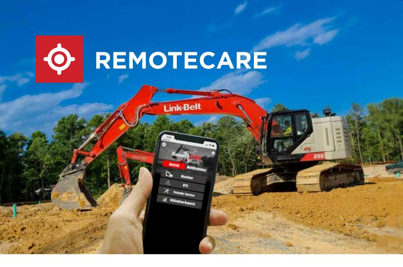
The 355 X4S comes standard with a new dual-band modem to improve RemoteCARE communication and functionality with greater range and real-time data capabilities. With 24-hour RemoteCARE®, you'll always know the hours, location, performance, diagnostics and security status of your equipment. Proactively monitor, plan and address preventative maintenance items, receive machine health notifications via email, and review average fuel consumption rates for your machine right from your smartphone.
