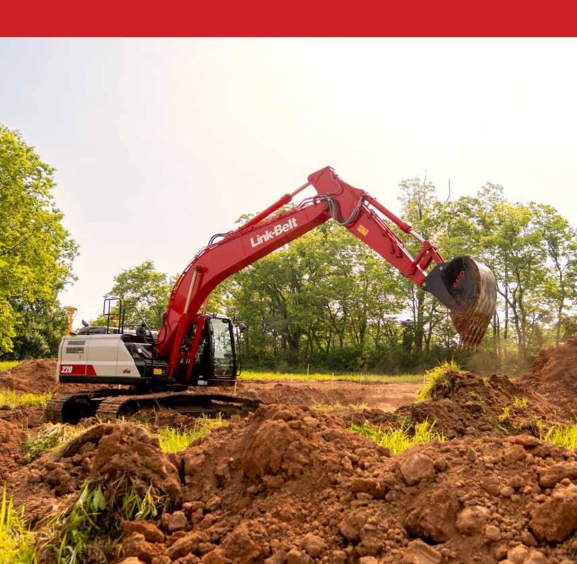
**SAE Net Horsepower** 160 hp (119.3 kW)
