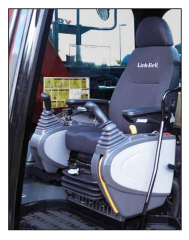
The X4 Series offers the most advanced and roomiest cab in its class. Comfortable, automotive-grade high-back seat with head rest provides superior lumbar back support. With a longer and wider seating surface, it reclines to a 155° maximum reclining angle to create a relaxed environment during breaks. Air-suspension seat is standard with tilting adjustment and seat heaters available as options.
