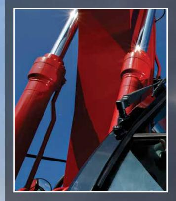
Greater digging power, increased lift capacities and faster cycle times start with our intuitive Ulti-Flow™ hydraulic system featuring a 30% larger hydraulic passage area, larger spools and advanced controls. Pilot pressure sensors detect the type of work being done-such as digging or leveling-and then relays that data to proportional solenoid valves that quickly determine where optimal hydraulic pressures should be directed for that operation.
