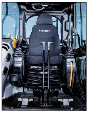
The X4 Series offers one of the most advanced and roomiest cabs in its class. Comfortable, automotive-grade high-back seat with head rest provides superior lumbar back support. With a longer and wider seating surface, it reclines to a 155° maximum reclining angle to create a relaxed environment during breaks. Air-suspension seat is standard with tilting adjustment and seat heaters available as options.
